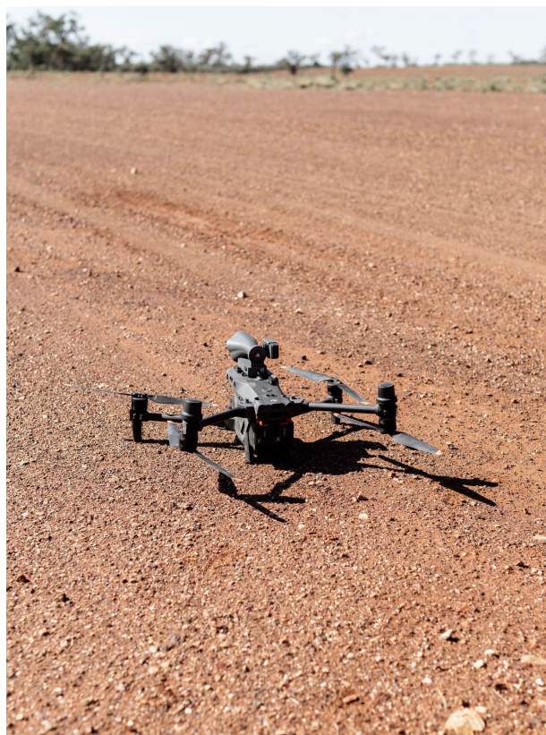
Figure 2. The DJI Matrice 30T drone fitted with thermal imaging and a loudspeaker attachment.
